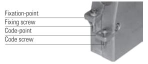
To code the TRAC F connector code screw at the connectorhood and code pins at the fixation frame are required. The coding of TRAC F connectors is preferably to be set during the final assembling, to avoid false coding configurations.
